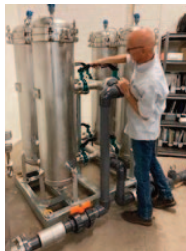
50 GPM Skid with single-bag prefilter and piping sub-assembly.
