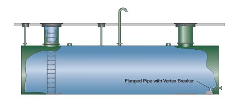
**Model HD-FPT-PW** - With a pump well for a vertical turbine fire pump. With this type of FPT, the fire pump impellers are fully immersed in the water, maintaining prime at all times.
