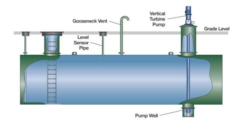
**Model HD-FPT-VS** - With a vertical suction pipe for use as an underground cistern to supply fire flow for fire department apparatus in a rural area.
