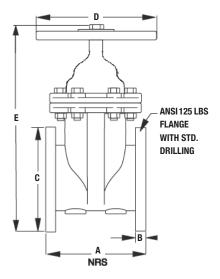
**APPLICATION:** Designed for installation on potable water lines, irrigation systems, waterworks connections and fire systems.
