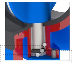
Thrust Bearing: Nylon Shaft Support.
