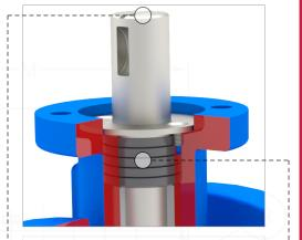
**Shaft**: Keyed one piece ASTM A276 type 316 stainless steel through shaft design providing minimal deflection. Slotted shaft top indicates position.
