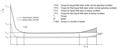
The motor power required to overcome the friction created by the interference fit of the rotor and stator on an Equal Wall stator is approximately 60% that of a Non-Equal Wall stator. This is a result of smaller surface contact.
