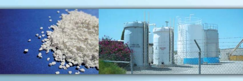
Activated alumina with its many types of adsorptive sites and high surface area is the perfect choice for the removal of contaminants from waters and to manage many remediation applications.
