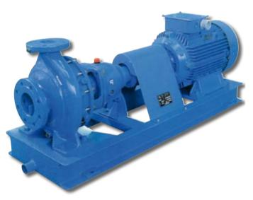
CN pumps are single stage centrifugal pumps, hydraulically balanced overhung impeller, simple volute casing, axial suction and radial discharge. Bearings are oil bath lubricated. The high standardization of the common parts simplifies spare parts storage. CN pumps are suitable for aggressive and viscous liquids. Particularly used in the chemical and food industries.
