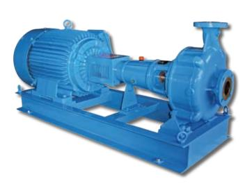
MCA pumps are suitable for pumping viscous and pasty liquids containing suspended solids thanks to the shape of the impeller and to its recessed position in the casing.
