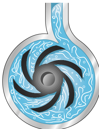
Typical Volute-Type Centrifugal Pump showing excessive turbulence and eddies
